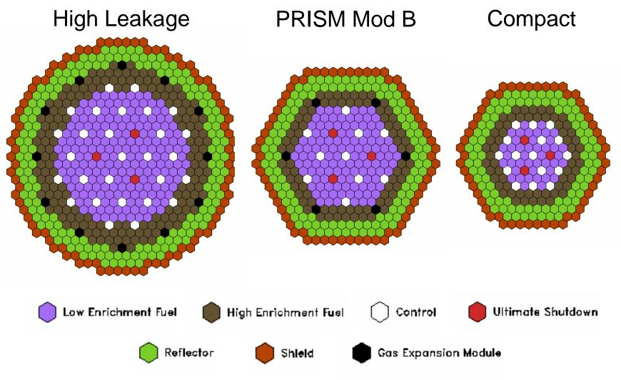
Fig. 8. Core configurations for several ABR candidates<sup>13</sup>
